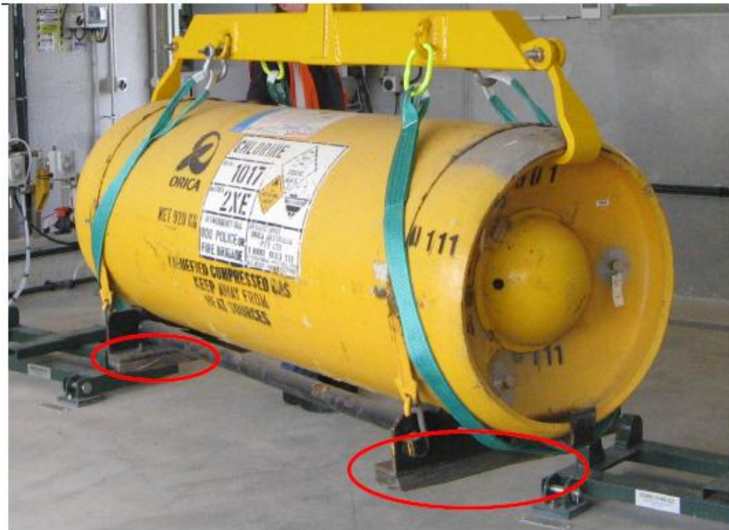
Liquefied chlorine drum transportation cradle base timber skids
