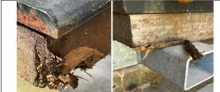
chlorine drum transportation cradle base timber skids examples of shredded or splintered timber
